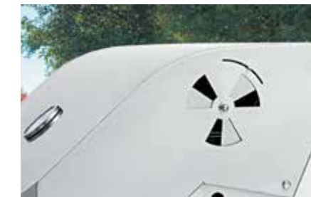
AIR/TEMPERATURE CONTROL LOUVERS
